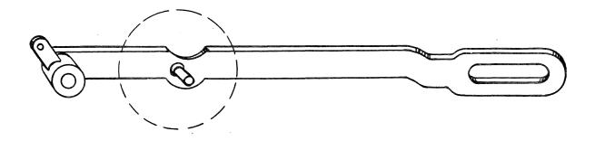
In making a field survey of the new Model 1015, we have found cases where the rivet on the actuating lever, shown above, is not tight.
